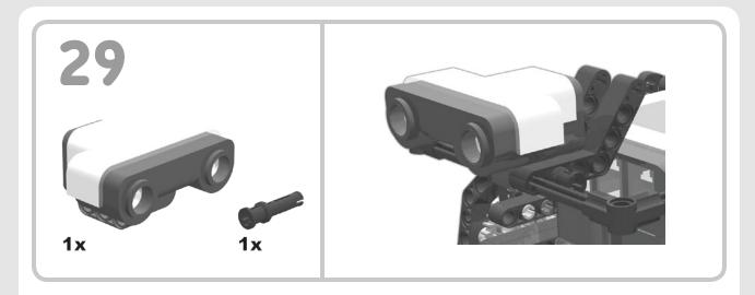
Place the sensor between the two bent beams. Thread the axle through the first hole in the sensor; insert a long pin into the second or third hole.
