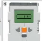
Select the port in which you have placed the Motor. Now try to attach a wheel to the Motor and measure the rotations by pushing the wheel over the floor.
