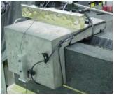
*References:* Vee & Flat bearings used on many common machine tools where gravity provides preload. NEAT uses two magnet tracks, one horizontal and one vertical, to provide horizontal and vertical preload force. Patent search revealed no other relevant art.
